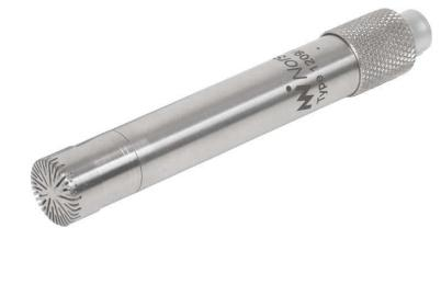
Adding the low frequency calibration shows this microphone has a hole in its diaphragm. Note it has normal responses at the 250 and 1k Hz frequencies used by sound calibrators so the problem would not be apparent in use. Would also give reasonable A weighted measurements.
